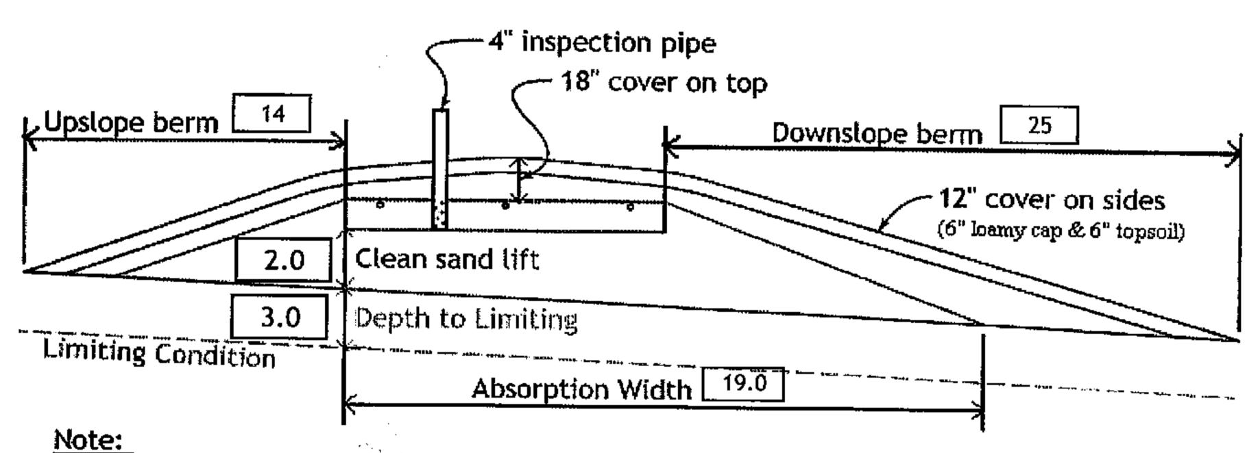
For 0 to 1% slopes, Absorption Width is measured from the Bed equally in both directions. For slopes >1%, Absorption Width is measured downhill from the upslope edge of the Bed.
